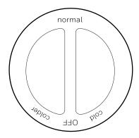
After powering on the cooler, you can turn the thermostat knob to set the inside temperature level.
