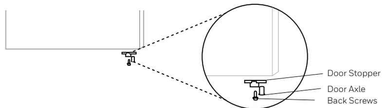
**03** Remove the door axle sleeve at the lower part of the glass door, door stopper back screws and door stopper, and fix them to the left side.
