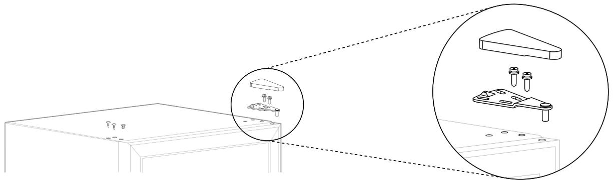
**05** Put the glass door on the lower hinge, install the door axle sleeve back and then install the upper hinge. Align the door with the cabinet and check the tightness of gasket.
