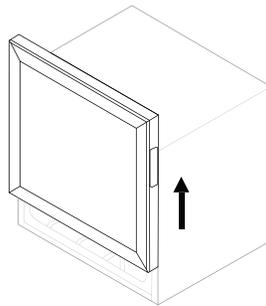
**02** Open the door of the beverage cabinet and detach the glass door with tremendous care.
