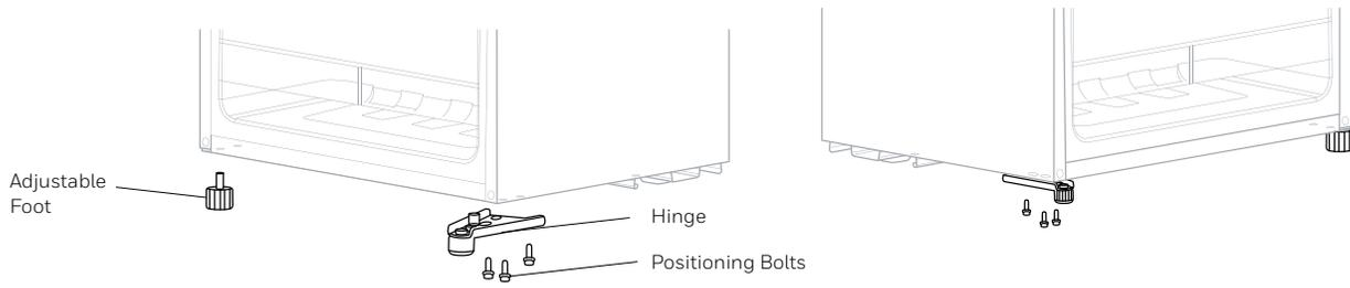
**04** Remove the adjustable foot, positioning bolts and lower hinge, then exchange the parts of right and left sides and later use the reverse method to install the adjustable foot and positioning bolts.
