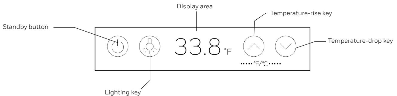
When powering on the cooler for the first time, the display screen will display in full for 3 seconds and the start-up tone will ring, and then the display will enter a normal running state.
