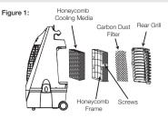
Removing the Carbon Dust Filter\*/ Honeycomb Cooling Media:
