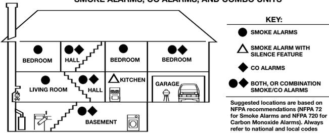
**In new construction AC and AC/DC smoke alarms MUST be interconnected to meet NFPA recommendations.**
