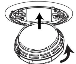
**NOTE:** Once the Smoke/CO Alarm is snapped onto the mounting bracket, you can rotate the Smoke/CO Alarm to adjust the alignment.
