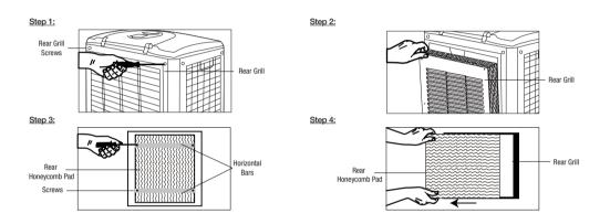
Removing the Honeycomb Cooling Media:
